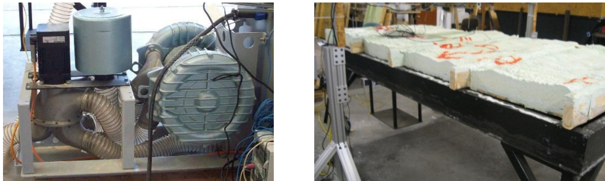
Figure 2. PLA (left) and panel loaded upside-down in pressure chamber (right).
