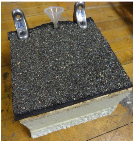
Figure 11: 6”x6” samples representing typical roof conditions
