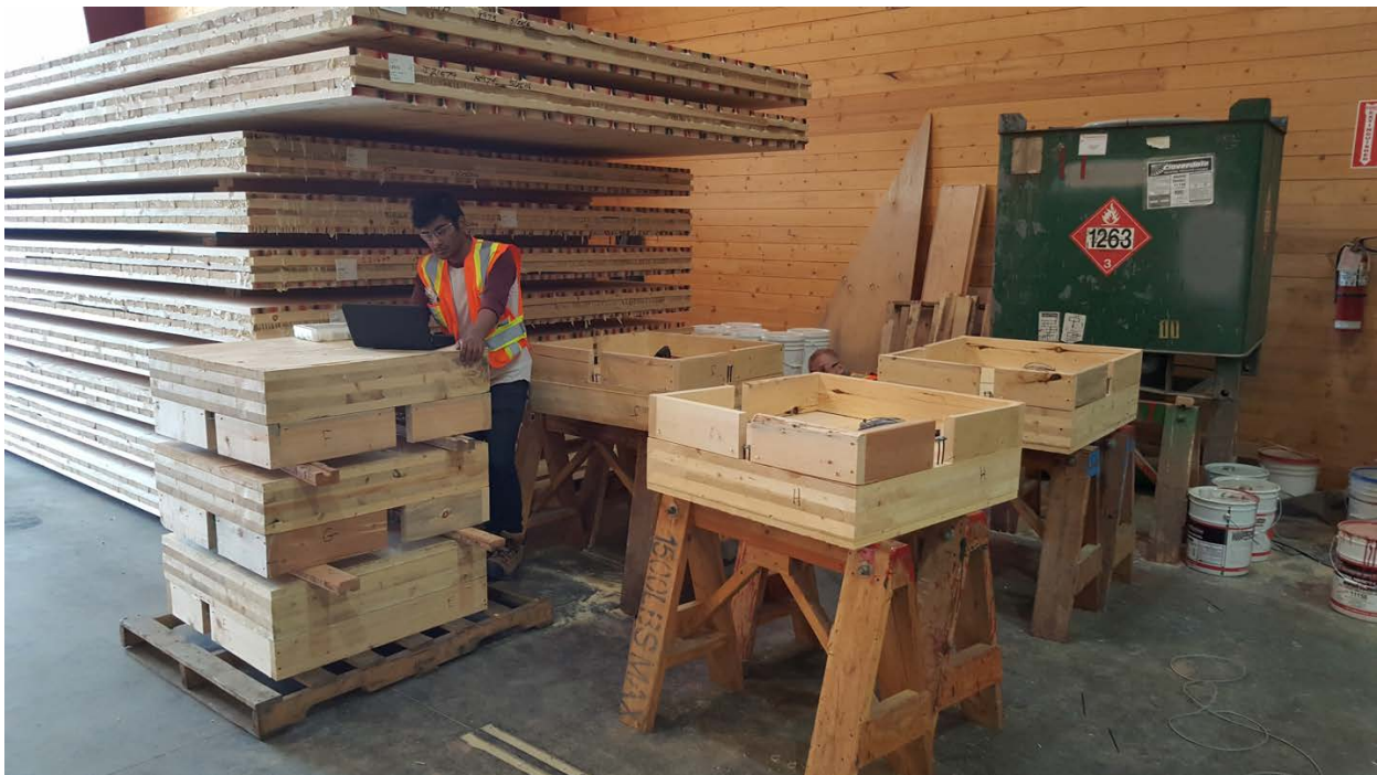
Figure 1. Installation of moisture probes in panels at Structurlam
