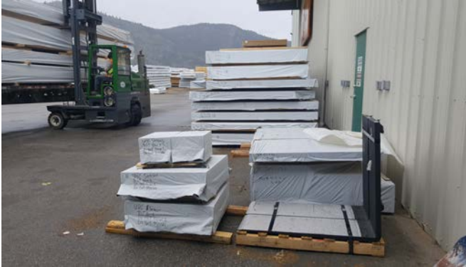
Figure 3. Covered panels monitored during storage at Structurlam Factory
