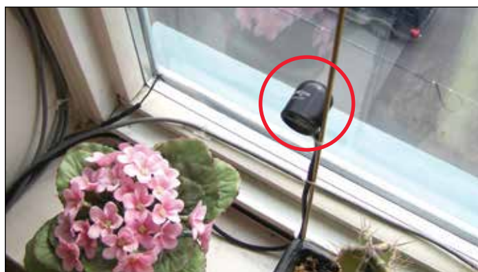
Figure 4 Pyranometer installed behind the fixed glazed portion of the HSG apartment bedroom window, facing outward (red circle).
