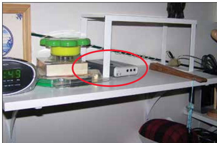
Figure 3 Data logger measuring indoor air temperature and relative humidity, typical installation (red circle).
