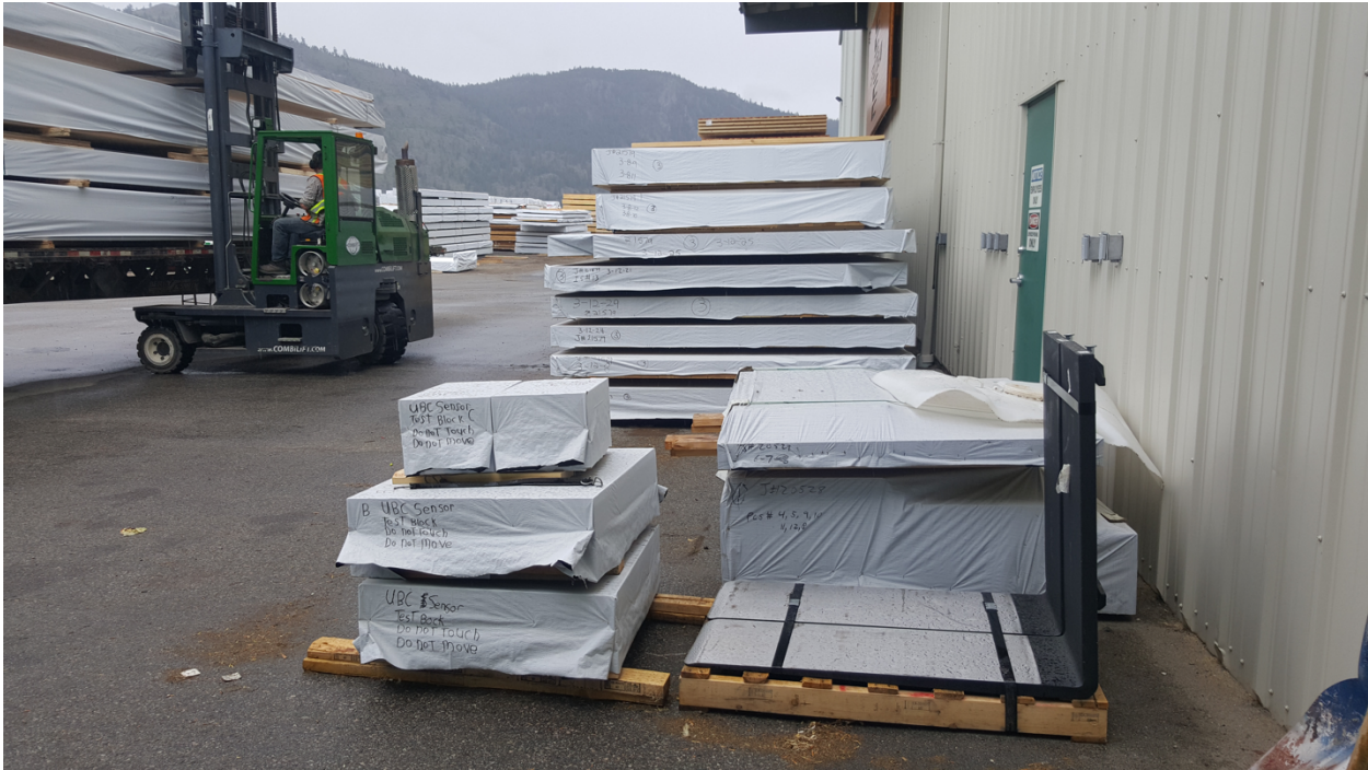
Figure 4: Off-cuts Stored outside alongside full size CLT panels
