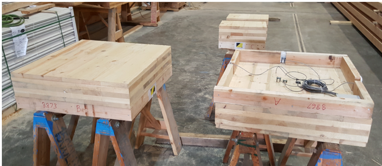
Figure 3: Instrumented Off-cuts – May 7th, 2016-06-01
