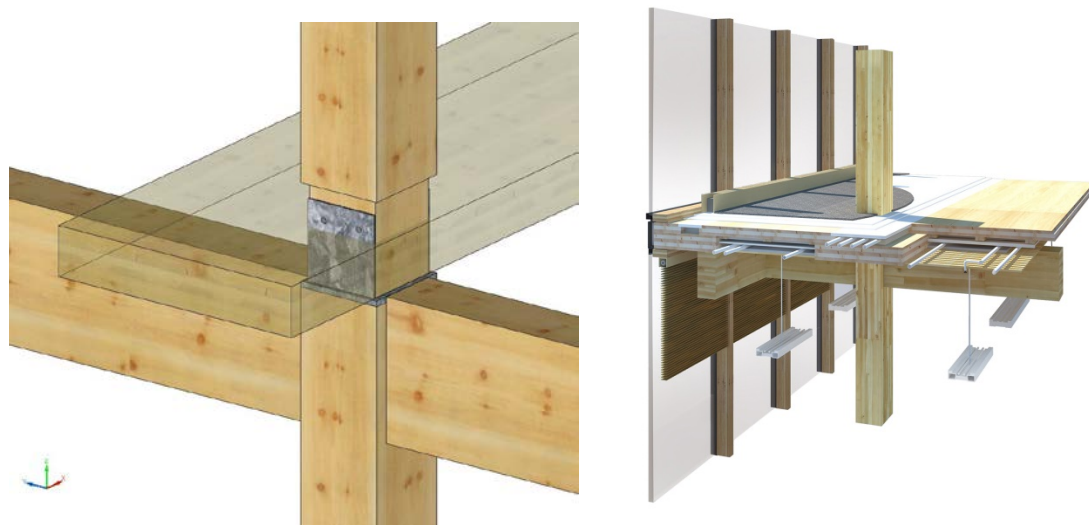
Figure 3 Left: Support of CLT floor slab with glulam column and beam (Courtesy of Equilibrium Consulting); Right: Vertically staggered CLT floor panels for providing chases to accommodate building services (courtesy of Michael Green Architecture)
