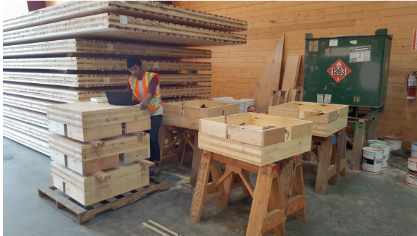
Figure 5. Six Additional Off-cuts Instrumented on May 27th, 2016
