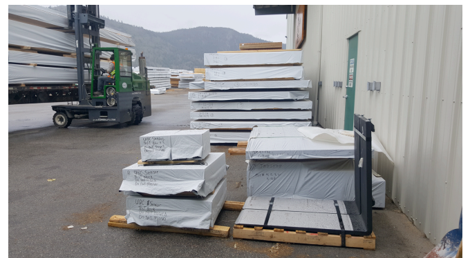
Figure 4. Off-cuts Stored outside next to Full Size CLT Panels
