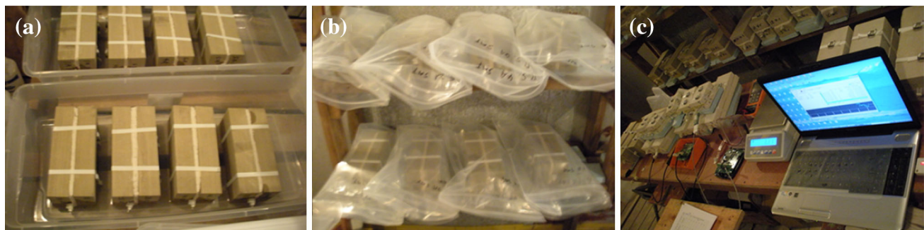
Fig. 5 Testing setup for the MC sensor calibration in a RH/Temperature controllable chamber
