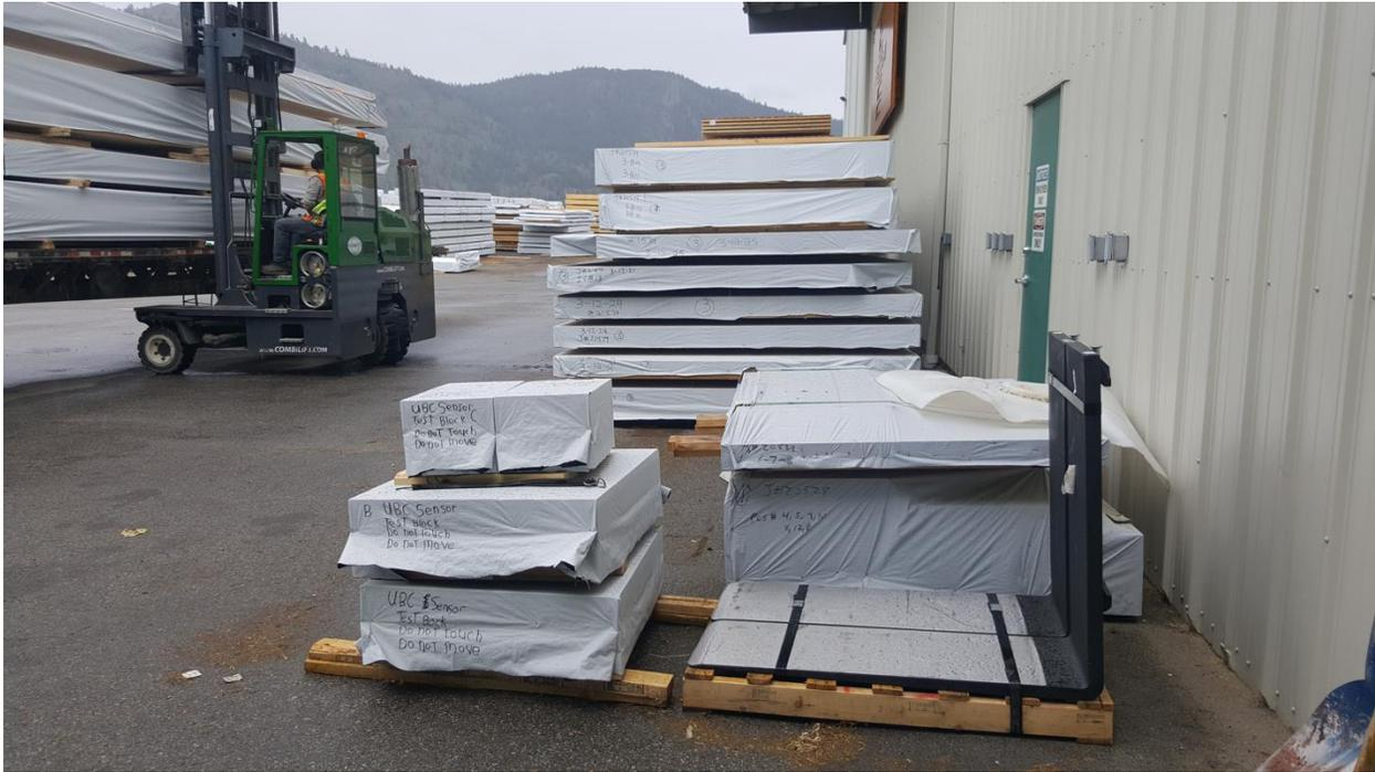
Figure 4: Off-cuts Stored outside alongside full size CLT panels
