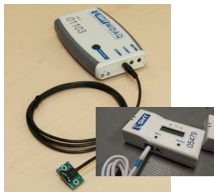
Figure 2. Plug audio jack into Mobile WiDAQ or A2. Screw into terminal blocks for Industrial WiDAQ and A3 models.
