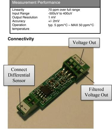
Connect the datalogger to the positive, negative and voltage out terminals.
