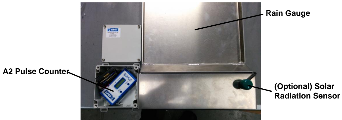
An example of a configuration for the Driving Rain Gauge (non-deployed). Has 1 of the 3 optional sensors available.
