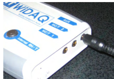
Figure 2. Insert audio jack into AUX port on the Mobile WiDAQ. BiG Input 5.
