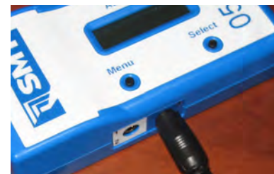
Figure 3. Insert audio jack into voltage port (inputs 3 and 4) on the SMT-A2 BiG Input 6.
