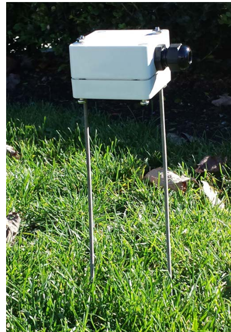
External CO 2 sensor monitoring grass
